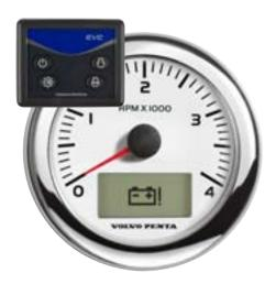
Standard instrumentation for D1/D2 consists of a start/stop panel and the tachometer with info display that gives you continuous readings of the rpm and engine running hours. Alarm symbols are in the display, with audible signals for low oil pressure, high engine temperature and low charge.
