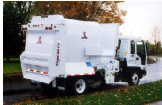
10 Yd Satellite with Cart Dumper and Upper Hopper Door
