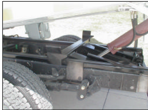
Rear Lift cylinder with body guides
