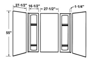
General: Furnish and install per plans, Stylemate® Bathtub Walls model 950, as manufactured by E.L. Mustee & Sons, Inc. The white thermoplastic wall system shall be 5-piece construction with four built-in shelves and seamless, overlapping corner panels.
