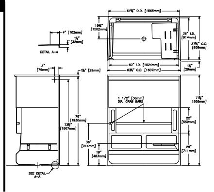
IMPORTANT: These dimensions are nominal and may vary within the range of tolerances established by ASME Standard A-117.1 and Z-124.2. The shower also complies with the guidelines issued by ADA, US Architectural and Transportation Barriers Compliance Board (A & T.B.C.B.) and with most city, state and national standards for barrier-free accessible shower facilities for the handicapped. Anti-skid floor treatment meets performance requirements of ASTM F462-78.
