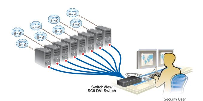
The NIAP Common Criteria certified SwitchView SC8 DVI switch supports eight secure channels, dual DVI-I video connections and lets you safely switch between computers operating at different classification levels, all from one keyboard, monitor and mouse.
