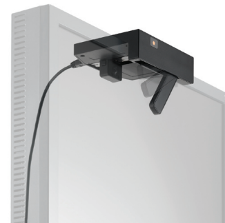
Figure 4. Sentry DX attachable remote network sensor
