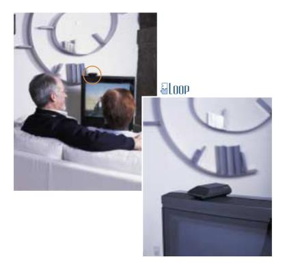
OOP is a teleloop amplifier designed to help users better hear the stereo and the TV. It can be used by anyone wearing a hearing aid with a T-position (telecoil) or using another inductive receiver. The sound from the stereo and/or the TV is transmitted directly to the hearing aid/inductive receiver so the user receives the sound clearly without interference from background noise, no matter how far they are from the sound source.
