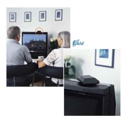
Wearing hearing aids with a T-position (telecoil) or for those using another inductive receiver. When the user's hearing aid is switched to T-position, the sound from the connected sound source is transmitted wirelessly from the teleloop system and picked up directly by the hearing aid - without any background noise.
