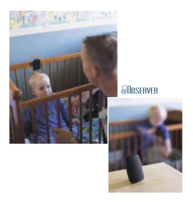
ith Observer, parents can safely put their child down for a nap, knowing that they will be alerted when their child awakens. Observer's microphone detects when the child cries and transmits that information wirelessly to one or more of the Puzzle receivers: Call, Flash, Wake, Pocketvib, Loop, Beam, and Link.
