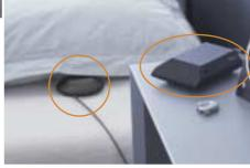
AKE is a vibrating alarm and alerting device which lets the user know when the alarm clock rings or when the smoke detector sounds by activating its powerful vibrator. Although WAKE plugs into an electrical outlet we do recommend using our battery backup in case of a power outage or an outage caused by fire.
