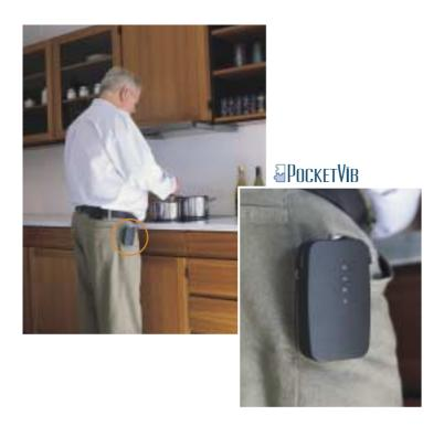
OCKETVIB is a small, powerful vibrator which receives alarm signals from the OBSERVER baby alarm and pager as well as from the doorbell, telephone, smoke detector, or other alarms using the DETECT alerting transmitter.
