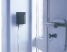
ALL is a sound alerting device which receives alarm signals from the doorbell, telephone, smoke detector, etc., via the DETECT alerting transmitter. CALL also receives alarm signals from the OBSERVER baby alarm and pager. When CALL receives a signal, its loudspeaker converts it into an audible sound signal.
