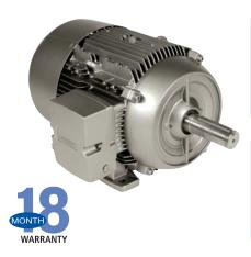
**Oversized Conduit Box** – Cast aluminum construction that is larger than industry standards, diagonallysplit and rotatable in 90° increments for quick and easy connections. Includes a ground lug and non-wicking, clearly and permanently marked leads.
