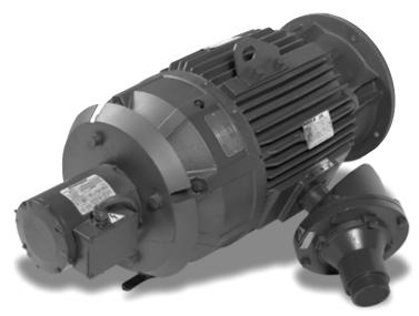
The totally enclosed blower-cooled immersible motor is equipped with a Reliance ½ hp motor for cooling. Once the motor is submerged, a float switch\* disengages the blower motor. The blower motor must be inspected and replaced if necessary before re-starting the motor dry.
