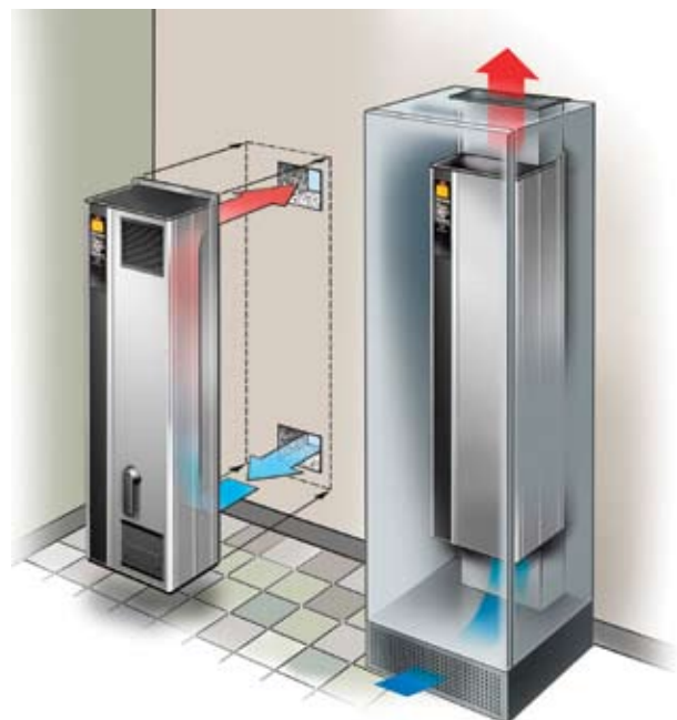
A smart, dedicated kit allows chassis/IP00 enclosures to be mounted in Rittal cabinets so cool air removes 85% of excess heat without contact with the electronics.
