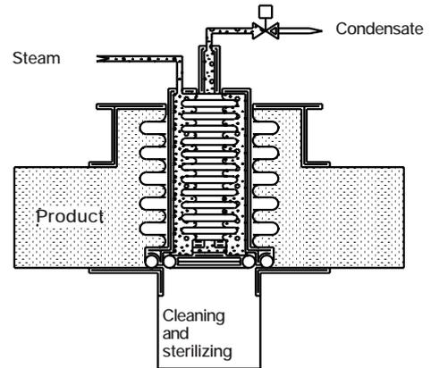
Fig.2.d. Barrier chamber sterilization.
