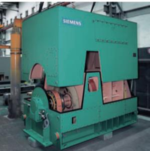
With the H-modyn, the main terminal box as well as the auxiliary terminal boxes are mounted on the motor baseframe, without any connections to the mounted cover with the integrated cooler. This means that the winding connections are decoupled from the cover, and the cover can be lifted without releasing the connections. The favorable ratio between the height of the baseframe and the mounted cover results in an extremely low installation and crane hook height.
