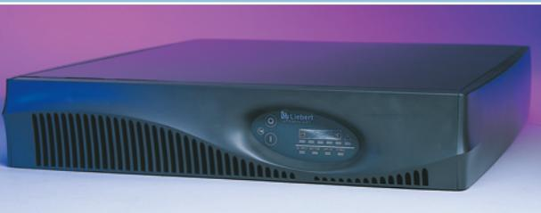
**Liebert UPStation™ GXT 2U True On-Line UPS System For Mission-Critical Power Protection** - A true on-line, double conversion UPS, the Liebert UPStation GXT 2U is available in sizes ranging from 500VA to 6000 VA. The unit's compact 2U size cabinet includes internal batteries and additional run time is easily added with external battery cabinets.
