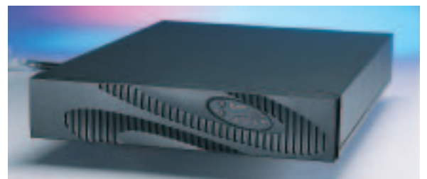
Your Liebert Foundation enclosure can also be bundled with the Liebert PowerSure® Interactive UPS. With its advanced line-interactive technology, this unit filters utility power to eliminate spikes, noise and other transients. It also contains a voltage “buck and boost” circuit that corrects input voltage — without switching to battery back-up.
