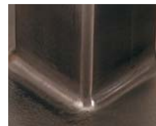
Group 3 Blended Weld
