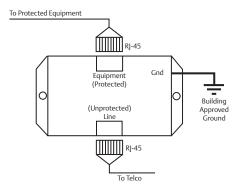
The Edco RJA and RJD Series are intended for indoor use only and shall be employed on the equipment side of a listed primary telephone protector.
