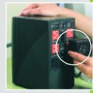
The PSA receptacles are spaced to accommodate transformer blocks.
