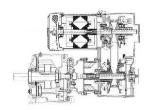
The CbN Varidrive includes selection of six beltcases, ranges of 4:1, 6:1 and 8:1; output torque to 145,000 in. lbs. and ratios from 1.6 to 6300:1. Motor available include single and three phase TEFC motors, CORRO-DUTY motors and explosion proof motors.
