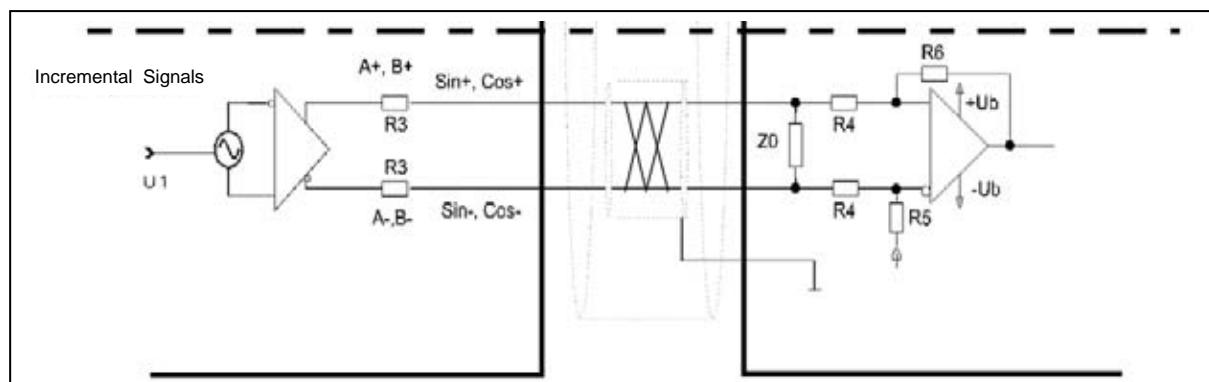
**2.5.6 Recommended input circuit with incremental track 1 Vpp**
