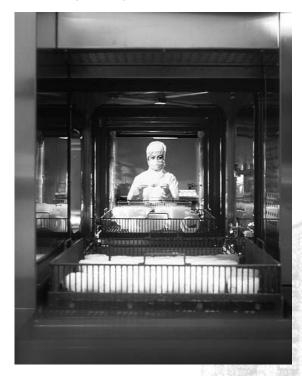
Fully automated 3-chamber cleaning system, precleaning with UPW/tenside, ultrasonic cleaning and final rinse with UPW ("all wetted parts" in PVDF and Halar), drying (hot air class 1000), 18.2 MΩ UPW.
