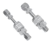
The HOKE Gyrolok Dielectric Tube Fittings are for use in applications where electrical current flowing through a pipe or tube line must be interrupted to protect vital instrumentation and metering equipment.
