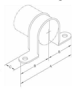
\* Hardened hex head self threading screw is furnished with the product and is the minimum fastener size acceptable.
