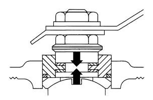
The R8 offers a stem that is inserted from inside the body cavity, is adjustable and self containing.
