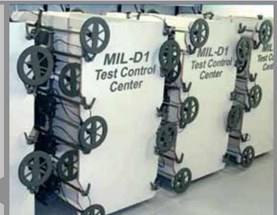
Operational test after assembly: 168 hours of continuous operation
