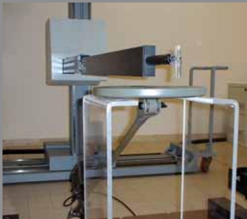
A metal detector antenna measurement being performed by a triple-axis robot.
