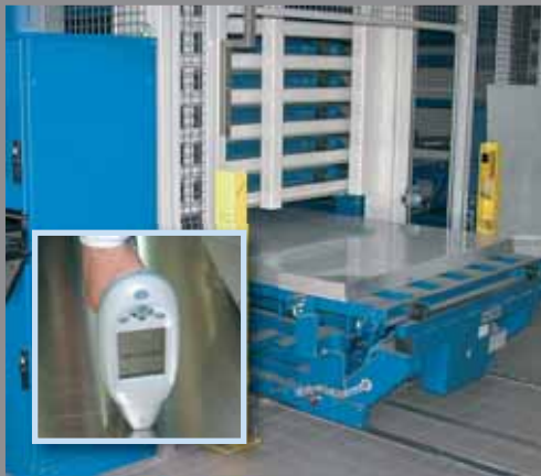
Incoming AISI 316L sheets check
