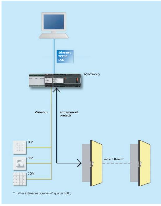
In conjunction with door controller IP, the Siedle access control system is capable of complying with high-level specifications in medium-sized buildings. While in terms of its price, input and complexity, the system remains easily manageable, its functional versatility extends to the field of professional access control requirements. The Ethernet interface and integrated Webserver make this a universally applicable system.
