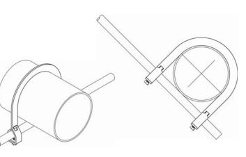
Component of State of California OSHPD Approved Seismic Restraints System
