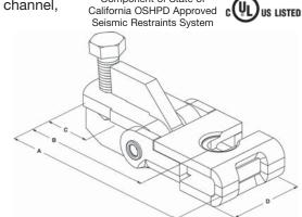
torque. Tighten existing hex nut down until the slight gap in the yoke assembly closes completely.
