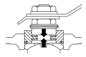
The B8 offers a stem that is inserted from inside the body cavity, is adjustable and self containing.
