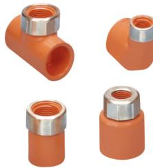
Spears® patented special reinforced (SR) plastic female thread design is one of the most significant advancements in the use of CPVC fire sprinkler system threaded fittings. Not just an added ring, this unique precompression design compensates for expansion forces generated from tapered pipe thread joint makeup. Radial stress is no longer a problem in normal installations and easily managed in severe over-tightening situations.
