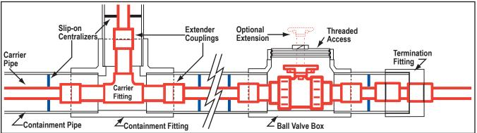
Carrier fittings are equipped with special extender couplings for connection to carrier pipe. Simple, slip-on centralizer brackets used on the carrier pipe support this assembly inside the containment pipe. This design allows the carrier fitting to "float" within the containment fitting, allowing ease of movement for installation while reducing problems associated with thermal expansion and contraction during operation.
