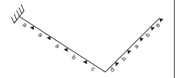
\* For example: If continuous support span is 10 ft., c + d must not exceed 7.5 ft. (c = 3 ft. and d = 4.5 ft. would satisfy this condition).
