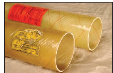
Old vs New - Pipe in the foreground was installed in 1973 and removed 27 years later when the station closed.
