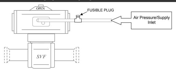
The SVF ESD (Emergency Shut Down) device is a heat actuated fusible plug that is installed as a Tee assembly into the supply air line to a pneumatic Spring Return actuator.
