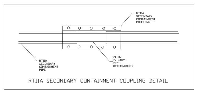
In order to achieve maximum flexibility of the RTIIA piping system, a secondary containment coupling should be used between dispenser sumps.
