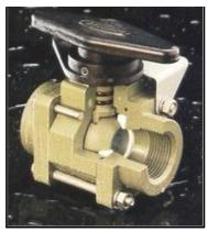
This special purpose ball valve is available in  $\frac{1}{2}$ ",  $\frac{3}{4}$ ", 1", 1 $\frac{1}{2}$ " and 2" sizes for corrosive chemical service in pressure piping systems. It is available in both Nil-Cor 510 (glass fiber reinforced PPS resin) and Nil-Cor 410 (glass fiber-reinforced polysulfone resin). Short term exposure to 300°F is acceptable. Exposure above 325°F should be avoided.
