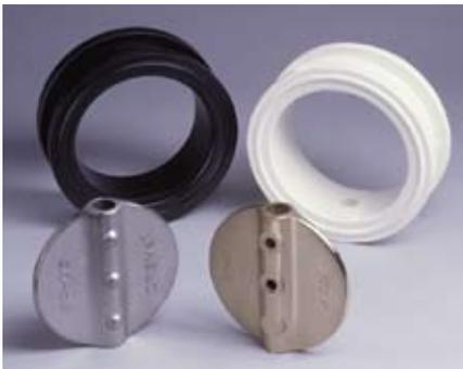
Discs are offered in Investment Cast 316 Stainless Steel, Nodular Iron, Nylon Coated Nodular Iron, ENP/Nodular Iron, Aluminum Bronze and a variety of custom coatings. Standard Seats are EPDM, Nitrile, Buna and FKM. Nitrile and EPDM are available in FDA approved white.
