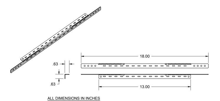
A versatile, galvanized steel bracket providing a platform for horizontal or vertical tube support. Also ideal for shower head, diverter, tub spout and sink applications.
