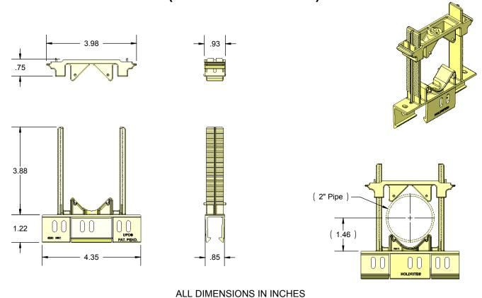
The HOLDRITE Stout Clamp™ #280-S is a fire retardant and smoke variable closure clamp. Clamp supports 1" to 2" CTS/IPS tubing sizes. Supports Copper, PEX, CPVC tubing, conduit, etc. Material meets ASTM E-84 25/50 and UL94V-0 fire rating.
