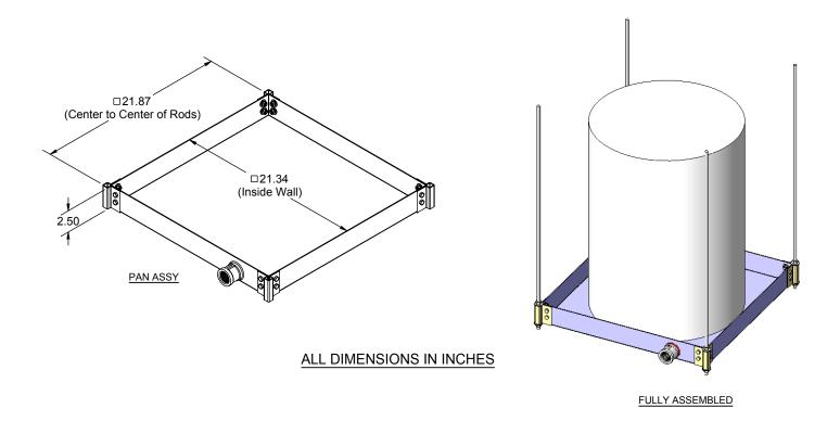
The Suspended Water Heater Platform is engineered to support water heaters up to 20 gallons (up to 375 pounds total weight). This time and labor savings tool is designed for the Professional Contractor. Design features requested by plumbers are incorporated into a professional platform that can be suspended with all thread rod.
