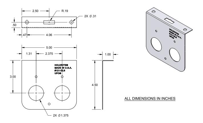
The HOLDRITE® #121-DLS is a 20 gage galvanized steel bracket that supports dual lines of 1/2", 3/4" or 1" Copper, PEX or CPVC tubing at 3" center line height. The hole pattern on the 90° base allows for attachment to any falt surface. The bracket can also be suspended by 1/4" or 3/8" threaded rod.
