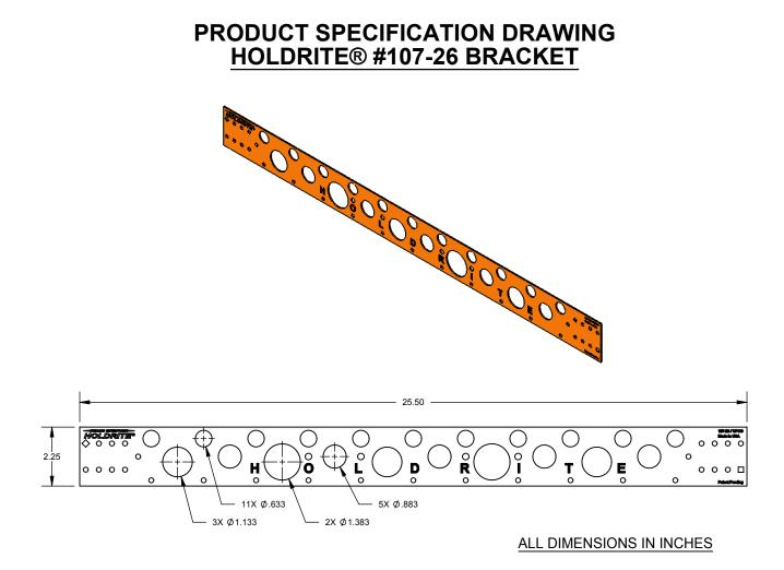
The HOLDRITE #107-26 is a Copper-Bonded<sup>™</sup> steel bracket with holes for 1/2" tubings on 2" centers, holes for 3/4" tubings on 4" centers, holes for 1" tubings on 8" centers, and holes for 1-1/4" tubings on 8" centers.
