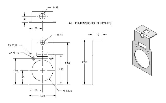
The HOLDRITE® #121-W is a 18 gage galvanized steel bracket with a 2" center line. The bracket will position 1/2", 3/4" and 1" Copper, PEX or CPVC for securing single tubing to any flat surface. The bracket can also be suspended by 1/4" or 3/8" threaded rod.
