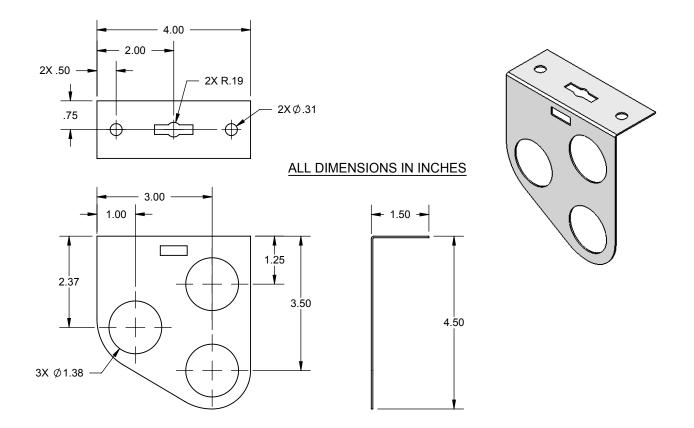
The HOLDRITE® #121-O is a 20 gage galvanized steel bracket that supports up to three lines of 1/2", 3/4" or 1" Copper, PEX or CPVC tubing. The hole pattern on the 90° base allows for attachment to any flat surface. The bracket can also be suspended by 3/8" threaded rod.
