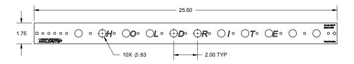
The HOLDRITE #101-26 are Copper-Bonded<sup>™</sup> steel bracket with 5/8" holes on 2" centers to support 1/2" copper tubing. The #101-26 position copper water supplies for sinks, water closets, and other fixtures. When soldering, heat the pipe, not the bracket.
