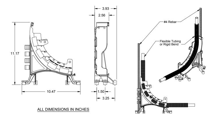
The PEXRITE® #708-E POP-UP<sup>™</sup> supports flexible pipe and tubing lines or rigid conduit up to 2" in a 90° pattern. Ideal for positioning pipe prior to concrete slab pouring. For elevated slabs, nail bracket to form decking or edge form. For slab-on-grade (ground work), secure bracket with #4 rebar driven into the ground.
