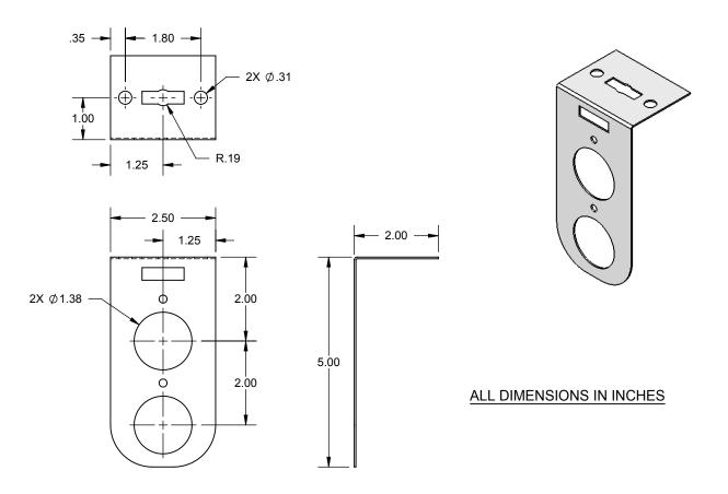
The HOLDRITE® #121-L is a 20 gage galvanized steel bracket that supports dual lines of 1/2", 3/4" or 1" Copper, PEX or CPVC tubing at 2" and 4" center line height. The hole pattern on the 90° base allows for attachment to any flat surface. The bracket can also be suspended by 3/8" threaded rod.
