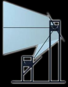
The OptaKong Mirror System is a rear projection mirror assembly, which facilitates the folding of projection image paths to reduce the amount of space required for rear projection installations. The OptaKong is also available with dual mirrors for increased reduction.
