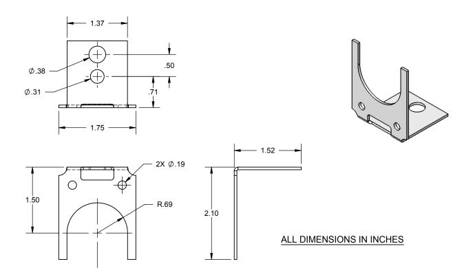
The HOLDRITE® #121 is a 16 gage galvanized steel bracket with an open "U" shape the secures single 1/2", 3/4" and 1" tubing.
