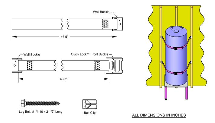
The QUICK BELT™ #QB-120-F is a seismic/earthquake support system for water heaters up to 120 gallons in size. The system includes: (4) Straps, (4) Lag Bolts and (2) Belt Clips. The Quick Lock™ system allows for secure locking of the strap from the front side of the water heater.
